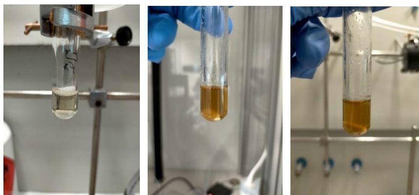
Figure 3.5. Solubility of PP in TBTDP DBS at r.t. (left), 80 °C (middle) and 250 °C (right)
